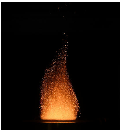
(a) A flat hybrid iron-methane-air flame stabilized on the perforated plate of the adapted HFB.
